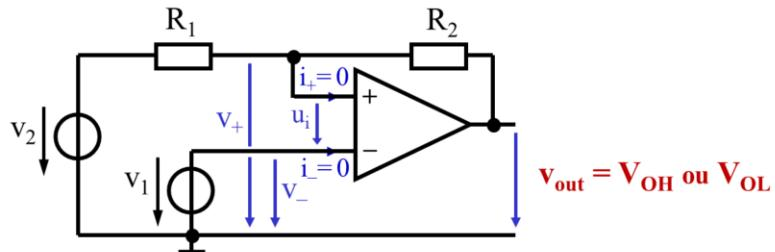
Superposition:  $\Rightarrow v_+ = \frac{R_2}{R_2 + R_1} \cdot v_2 + \frac{R_1}{R_2 + R_1} \cdot v_{\text{out}}$        $v_- = v_1$
